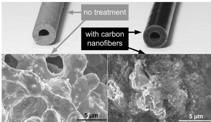
Figure 4.5: Porous stainless steel hollow fibers before (left) and after (right) the growth of the carbon nanofibers.
